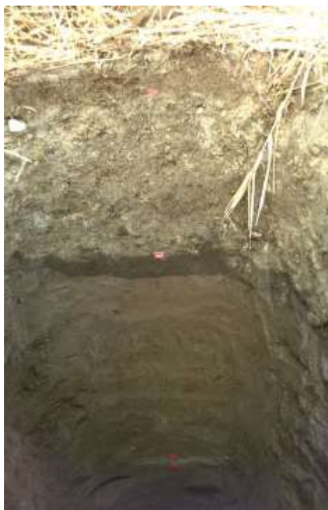
The soil pit pictures above show a dark horizon in the middle (left photo) and near the bottom (right photo) of the soil profiles respectively. This dark horizon is the “top soil” of the original meadow, which has been buried by clay sub-soil from the construction project to install the sewer pipe. The ground level was raised by around 50 -80 cm on the floodplain. The grey coloured “fill” is more compacted than natural soil and has very poor fertility.
