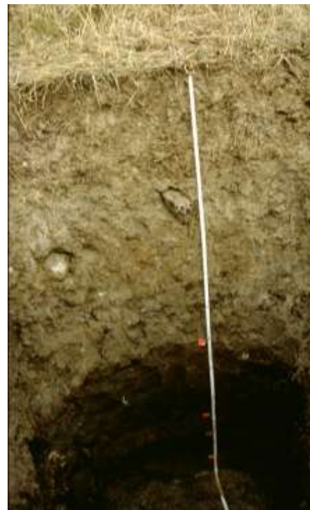
The soil pit pictures above show a dark horizon in the middle (left photo) and near the bottom (right photo) of the soil profiles respectively. This dark horizon is the “top soil” of the original meadow, which has been buried by clay sub-soil from the construction project to install the sewer pipe. The ground level was raised by around 50 -80 cm on the floodplain. The grey coloured “fill” is more compacted than natural soil and has very poor fertility.
